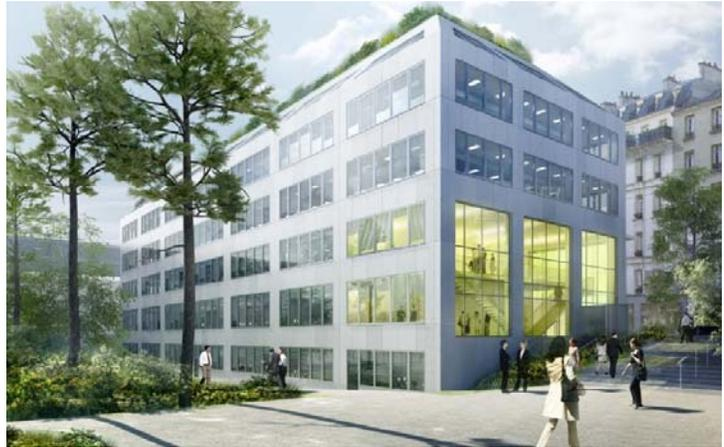
Green One is a four-story office building with a garden level and a ground floor. The building structure is compact with external wall insulation and facades made of concrete resin panels. Double glazing was used except on the south side of the building where filtering glazing was chosen. There is a flat roof with a small solar photovoltaic glass roof.
