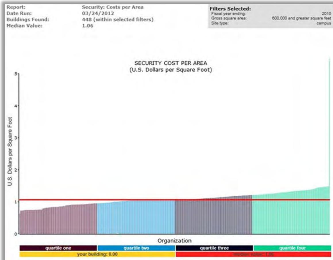
Figure 13. Security cost per unit area for large buildings (>600,000 sq. ft.) in a campus-setting (multiple buildings).
