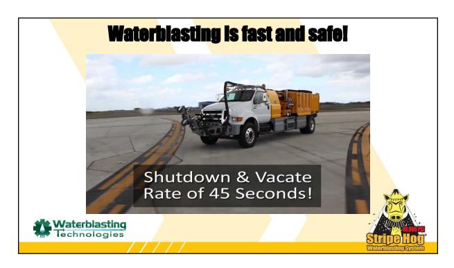
When a Stripe Hog is on a runway working whether removing a marking or runway rubber it can shut down and vacate the runway in 45 seconds in the case of an emergency landing.
